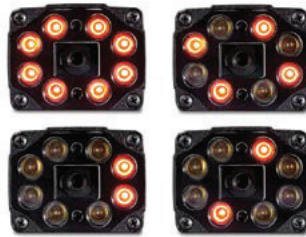
Independent lighting controls
